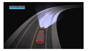
Figure 4 Adaptive steerable headlight system
