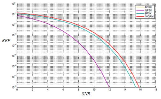
Fig.4 Comparative BEP Graph of BPSK and QPSK
