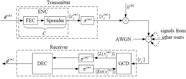
Fig.3 Transmitter and receiver structures of IDMA
