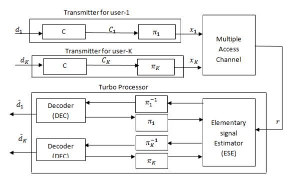
Fig.2 Transmitter and receiver structures of IDMA
