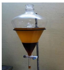
Figure 4(j). Separation after transesterification
