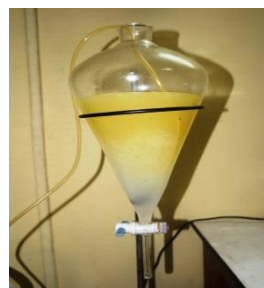
Figure 4(k). Water washing
