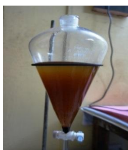
Figure 4(f). Separation after esterification
