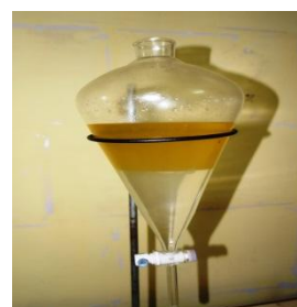
Figure 4(l). Separation of methyl ester and water
