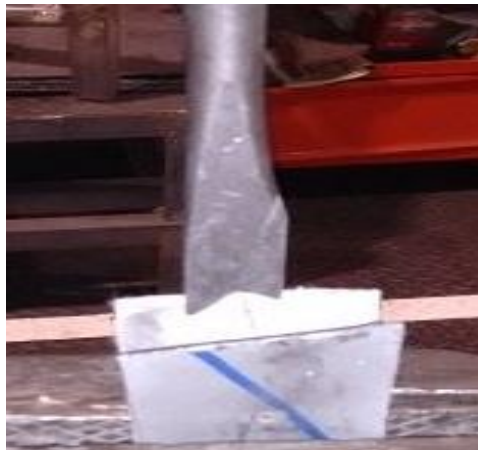
Figure.5: Destructive Peel off Test
