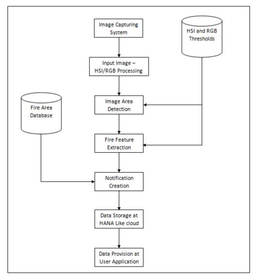
Figure 1: Block Diagram for the system
