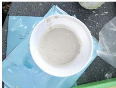
Fig 14: Plaster Of Paris is with water
