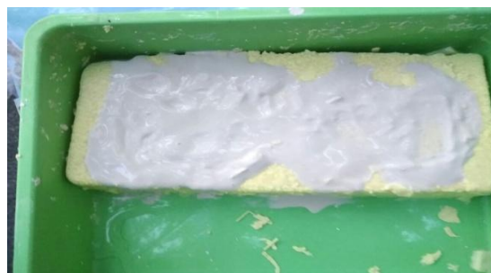
Fig 16: The Plaster Of Paris is poured into the pattern.
