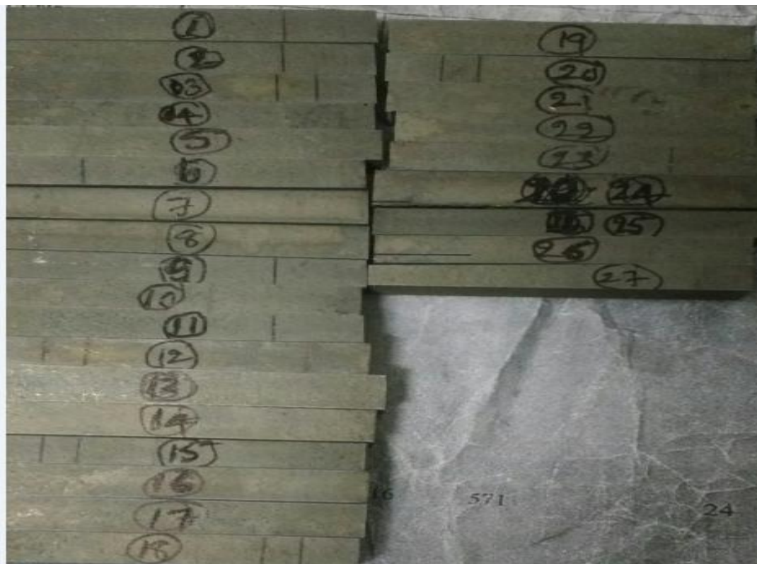
Fig.3. Cutting of Ti-6Al-4V as Per Taguchi L27 on Wire EDM
