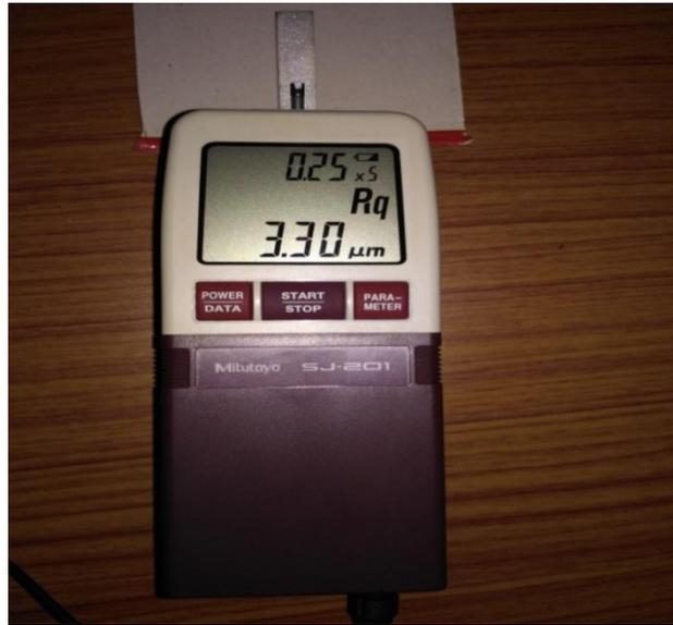
Fig.2.Mitutoyo SJ-201 Talysurf.
