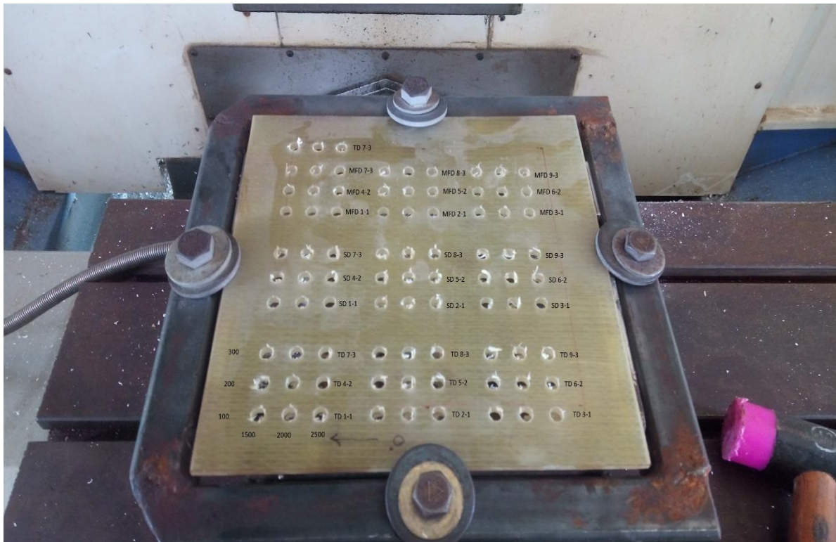
Figure 4 Drilled Laminate of GFRP
