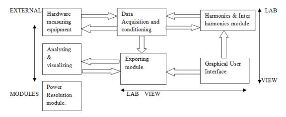
Fig: 2 Power Monitoring system
