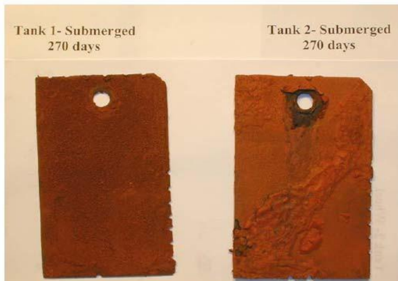
Corroded plates after 270 days exposure in submerged Environment.
