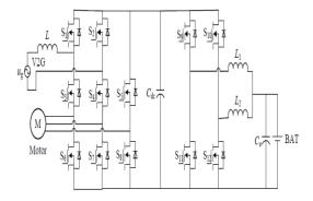
**Figure 3.** Topology of non-isolated integrated bidirectional charger composed of eight-switch inverter (ESI) and interleave DC-DC converter.
