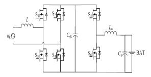
**Figure 1.** Topology of non-isolated on-board bidirectional charger composed of pulse width modulation (PWM) converter and bidirectional buck-boost DC-DC converter.
