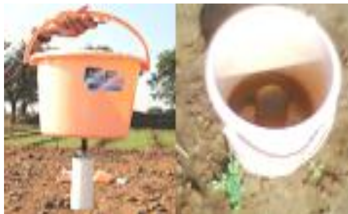
Fig. 1 Custom-made Porous Capsule Assembly
