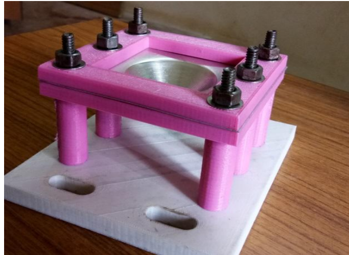
Fig.3 3D printed Fixture arrangement
