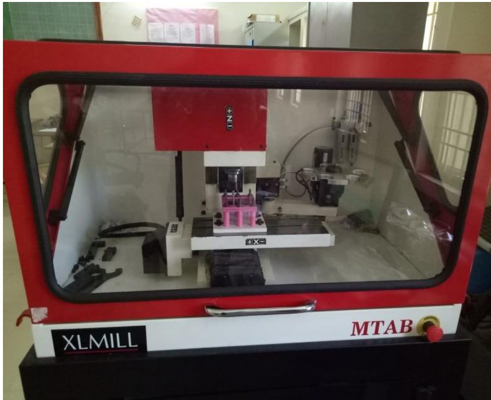
Fig.1 Experimental setup using CNC milling machine
