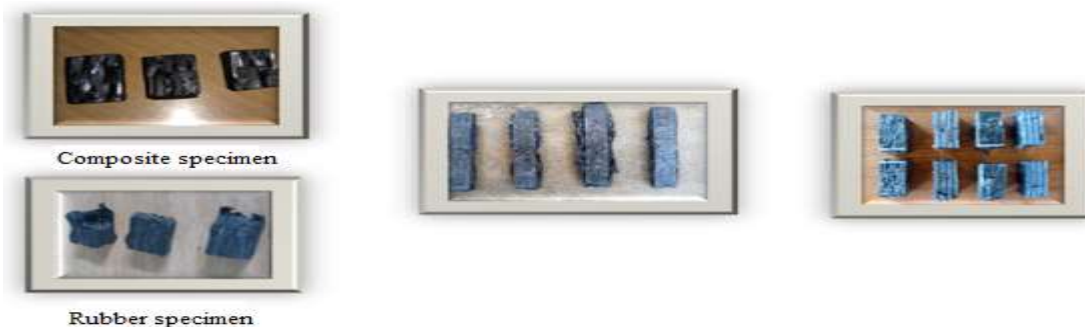
Figure 3. Specimens after testing for wear, compression and impact test respectively
