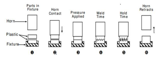
Fig. 1. Phases of ultrasonic welding
