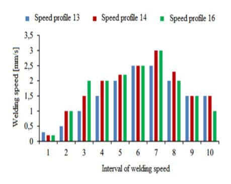
Fig. 3. The three best speed profiles exhibiting the highest joint strengths
