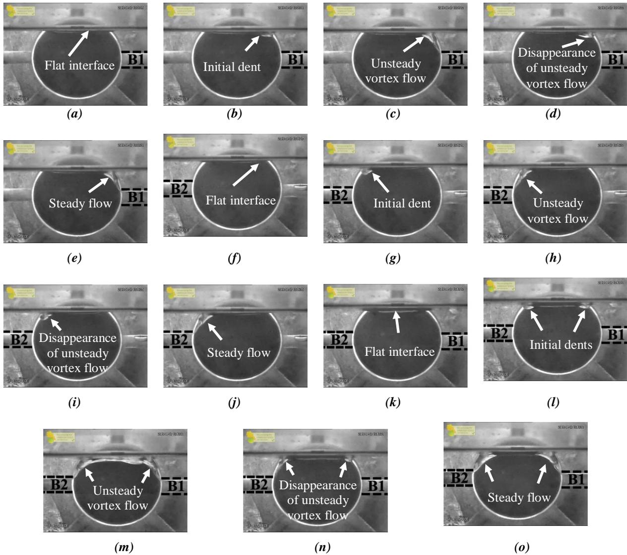
Figure 6 . Typical Gas entrainment phenomena for series nos. 1, 2, and 3
