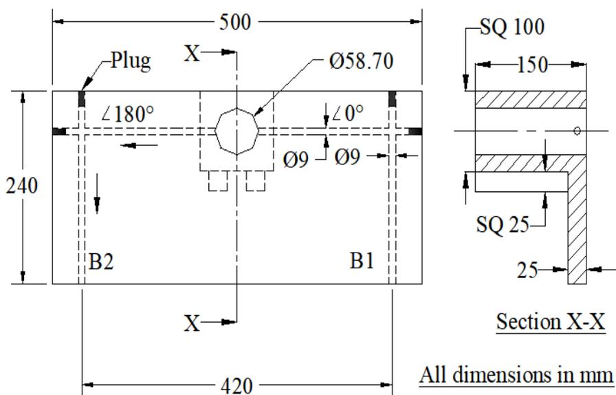
**Figure 4. Schematic of test piece**
