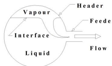
Figure 1. Schematic of typical PHWR header Figure 2. Vapor pull through phenomena
