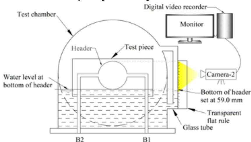
*Figure 5 Schematic of liquid level measurement*
