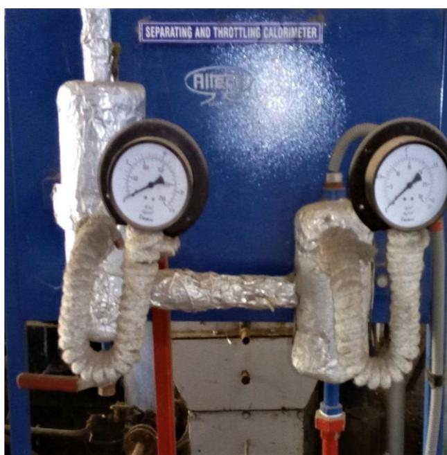
*Figure 4.1. Separating and throttling calorimeter*
