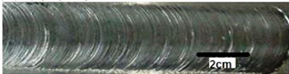
Fig 2 Surface morphologies of weld without defects
