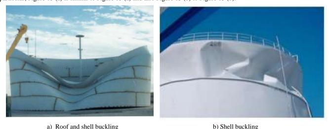
Figure 15 Buckling shape due to earthquake
