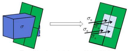
Figure 4 Normal stress in the intersected Euler cell [11]
