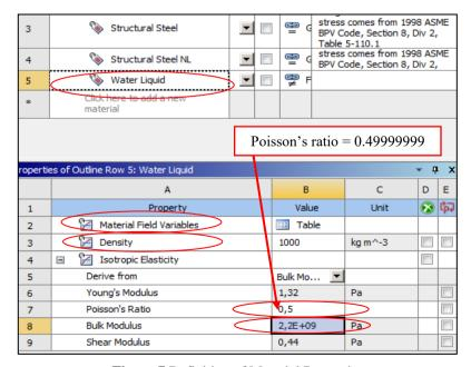
Figure 7 Definition of Material Properties
