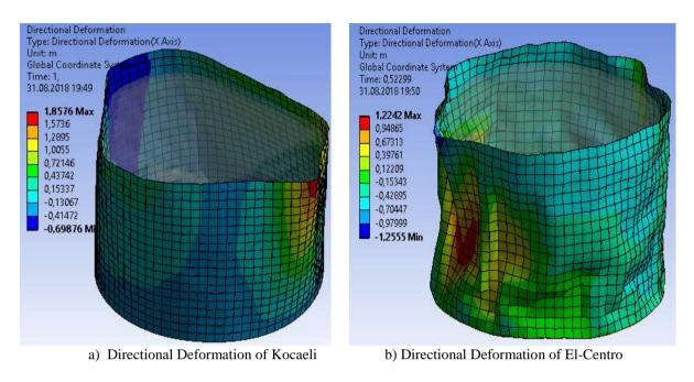
Figure 14 Directional Deformation of Open-top tank
