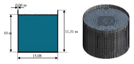
**Figure 1.** Design Size and Meshed View of Tanks
