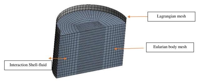
Figure 10 Mesh models of tanks
