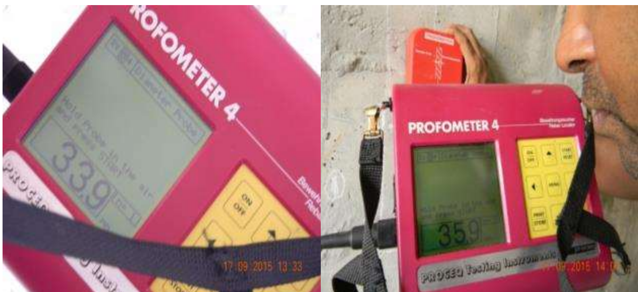
Figure-4.1 (a) A closer view of the Dia observations (b) Close view of the previous Rebars dia measurement
