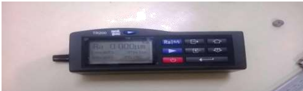
FIGURE 2.5: TR200 SURFACE ROUGHNESS TESTER WITH WORKPIECE
