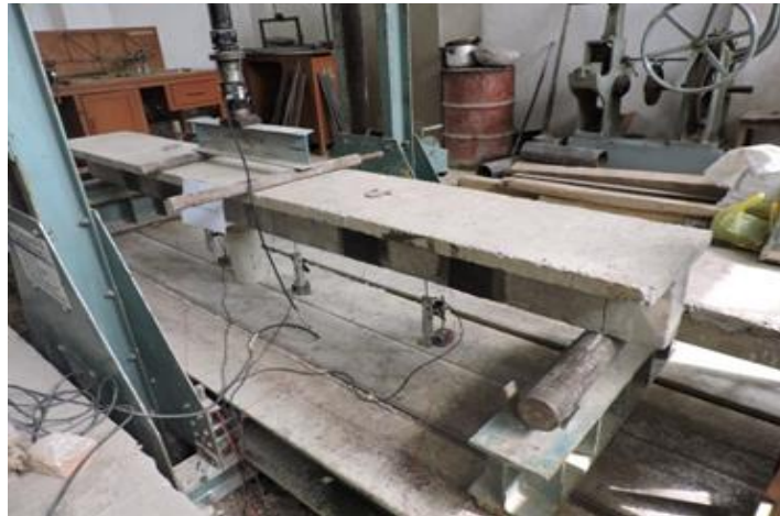
Figure 5. Test setup for T-shape girder model
