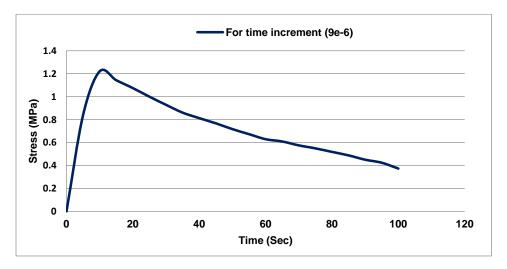
Figure 4 (b): Stress relaxation for time increment 9 x 10<sup>-6</sup> Sec
