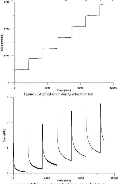
Figure 2: Resulting stress relaxation under applied strain
