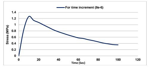
Figure 4 (c): Stress relaxation for time increment  $8 \times 10^{-6}$  Sec
