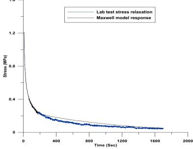
Figure 3: Maxwell model response to simulate asphalt concrete response
