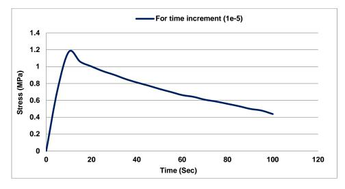
Figure 4 (a): Stress relaxation for time increment  $1 \times 10^{-5}$  Sec
