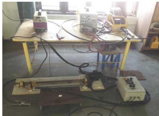
Figure 1: Automated TIG welding setup
