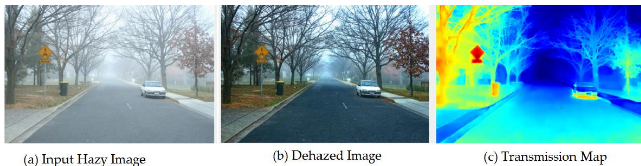
Fig2: Example of visibility improvement by applying the dehazing algorithm
