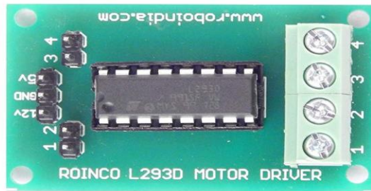
Figure 2: PWM Motor Driver Circuit
