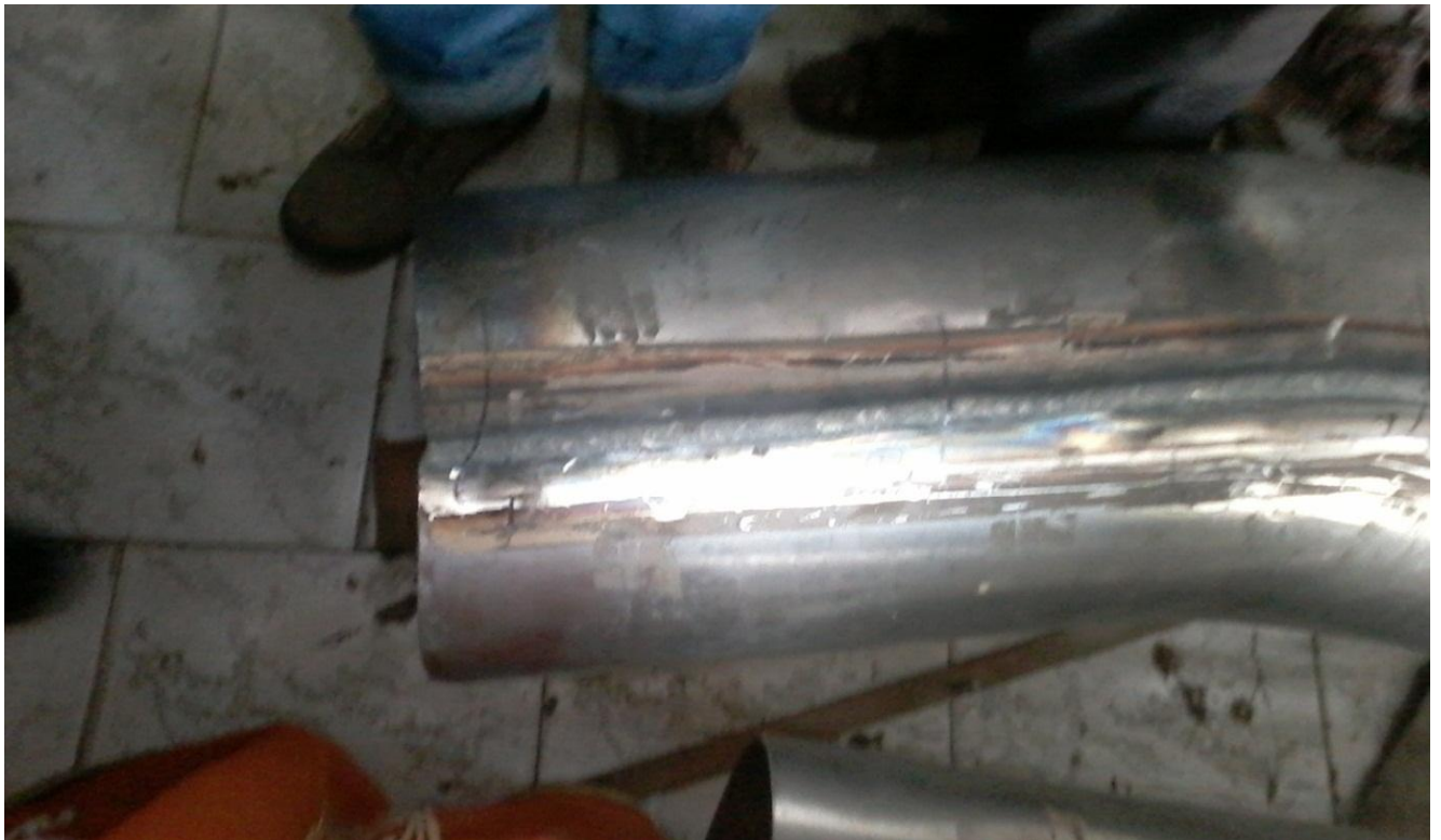
Figure: 5 Welded steel pipe (GAMMA Radiography Technics-HYD)
