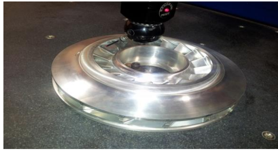
Fig 8. inspecting the shrouded impeller internally by using probe
