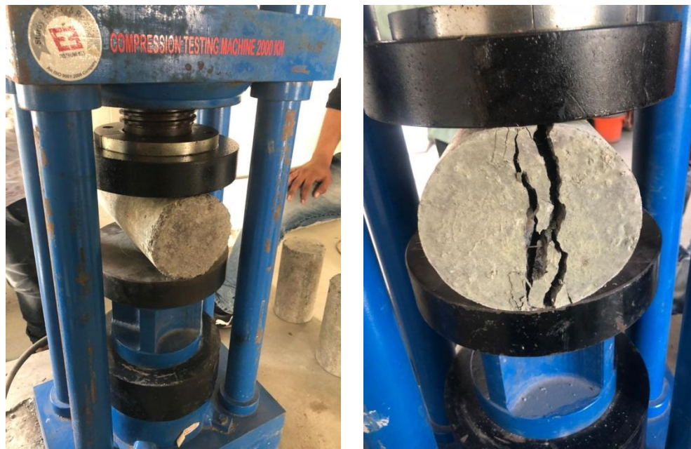
Testing of cylinders for split tensile strength
