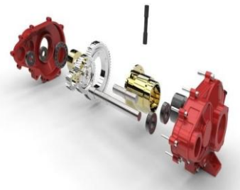
Fig 2: Exploded view of Gearbox
