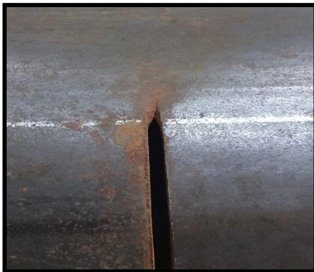
Figure 5 show the crack on pipe after test Figure 6 show the dimensions of pipe
