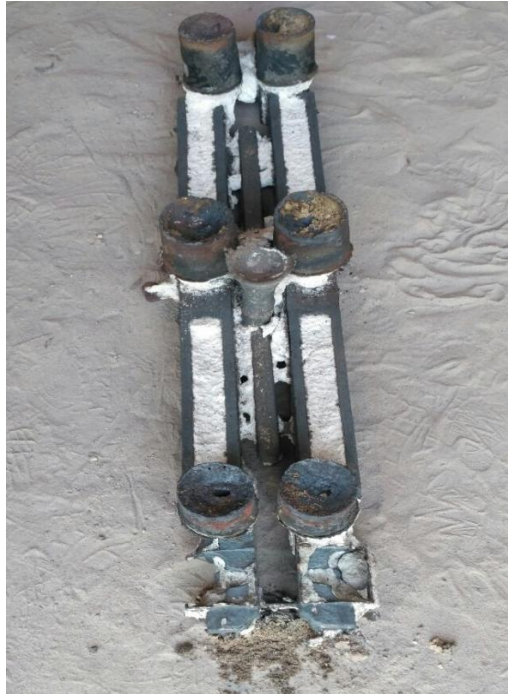
Figure 1(b). Flat bar casting with 6 risers and sprue
