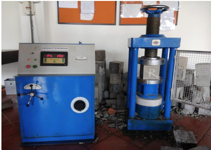
Figure: Compressive strength of cubes
