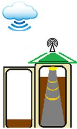
Figure 3. Sensors in the smart trash can
