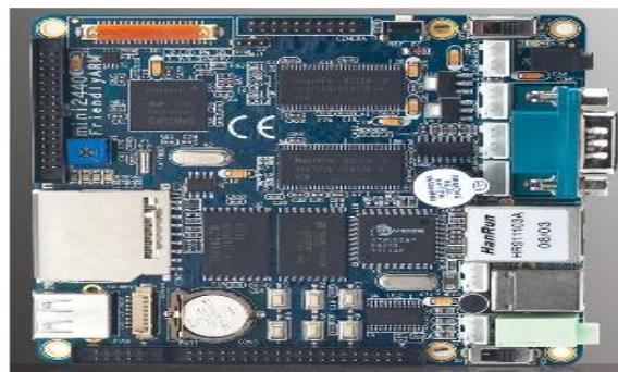
Fig5. Mini2440 Development board
