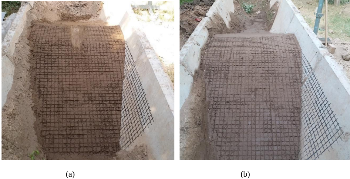
Figure 2.5. Illustration of the dam model placed in the channel (a) initial pilot channel provided at the middle of the crest (b) flat crest top level
