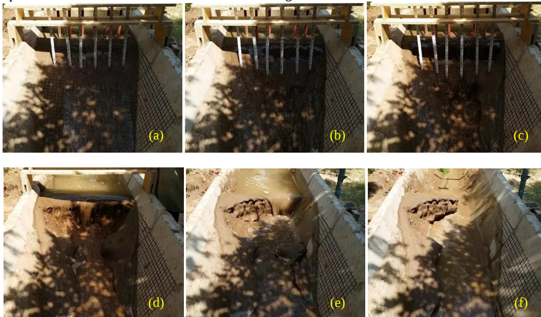
Figure 2.6. Breach development process (test 2): (a) rill and sheet erosion at t = 20 sec (stage-1), (b) formation of headcut at t = 85 sec (stage-2), (c) migration of headcut toward crest of embankment at t = 160 sec (transition from stage -2 to stage -3), (d) erosion of crest and clay core at t = 330 sec (stage-4) (e) headcut at upstream side (lowering of crest level) during stage-4 at t = 535 sec (f) complete failure at t = 845 sec.
