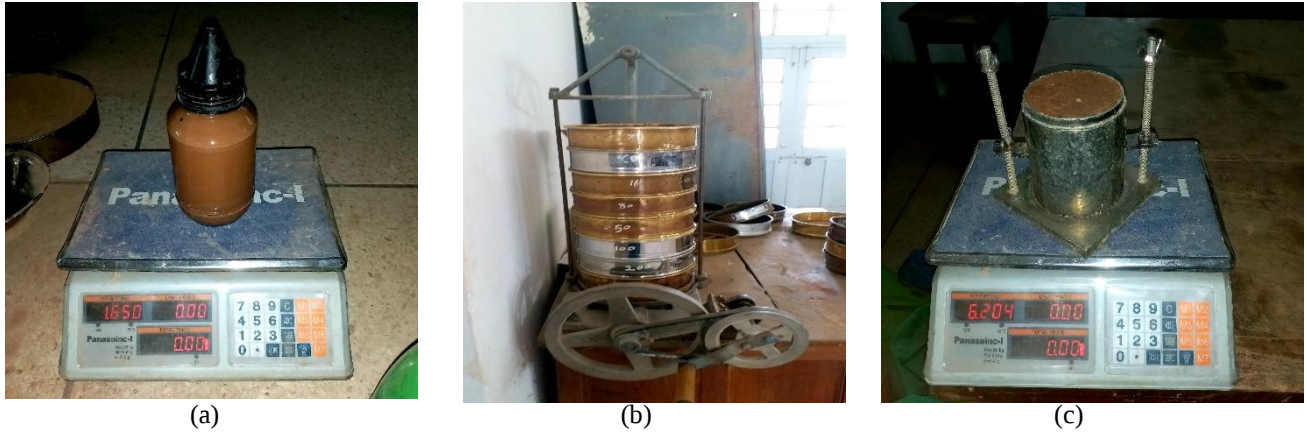
Figure 2.1. Laboratory tests of the selected soil samples (a) specific gravity test, (b) sieve analysis test, (c) standard proctor compaction test
