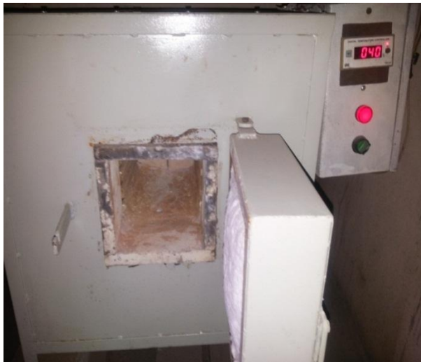
Ceramic fiber wool placed on door of Oven
