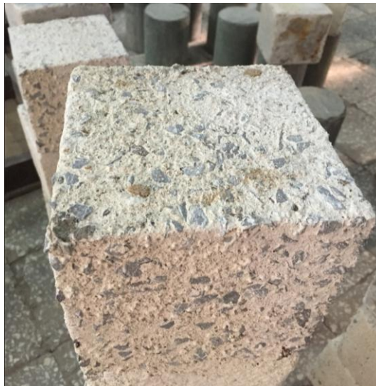
Figure 5 Acid Ponding Test
