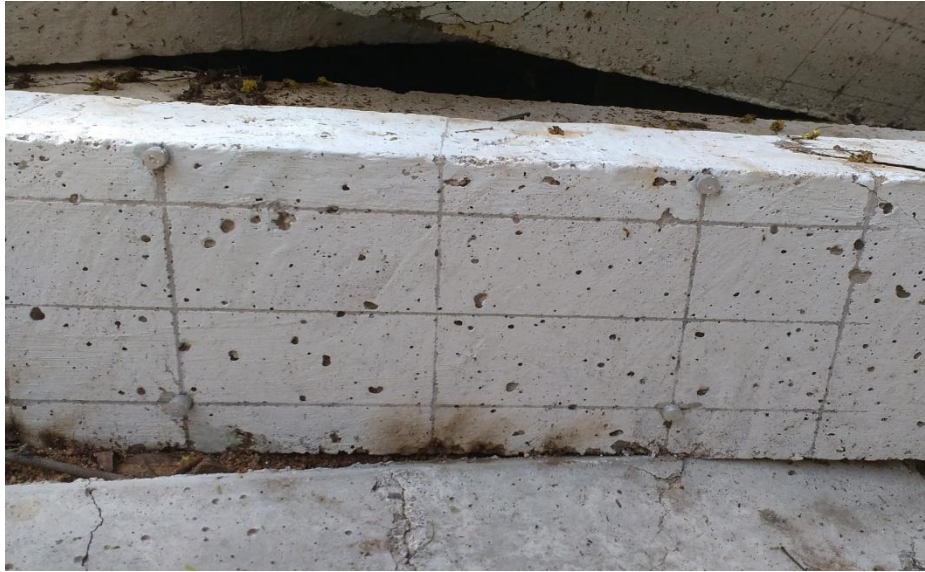
FIG 6 Pillets fixed for strain measurement
