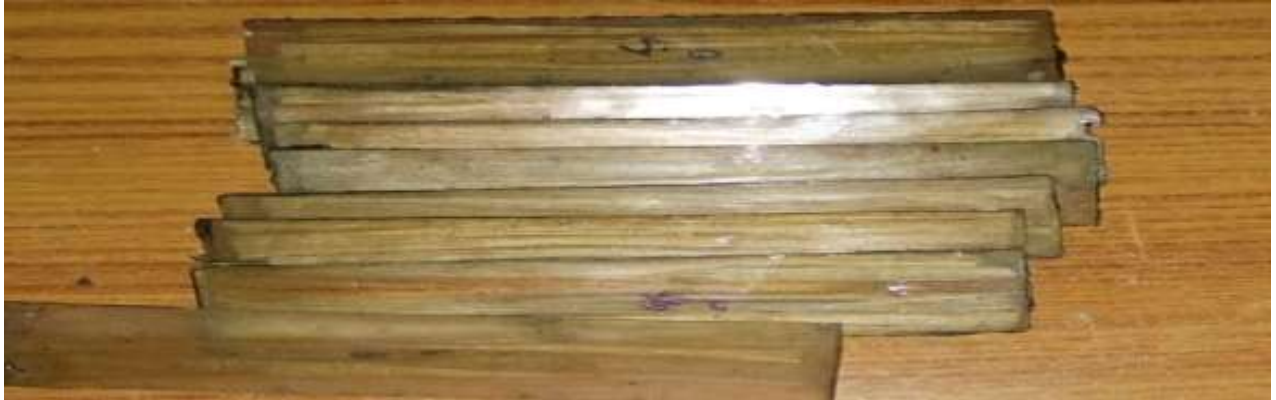
Fig.6 Flexural testing specimens
