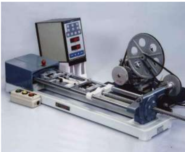
Fig.8 Electronic Tensometer for tensile testing of composites
