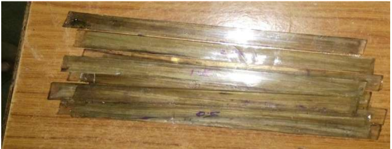
Fig.5 Tensile strength specimens
