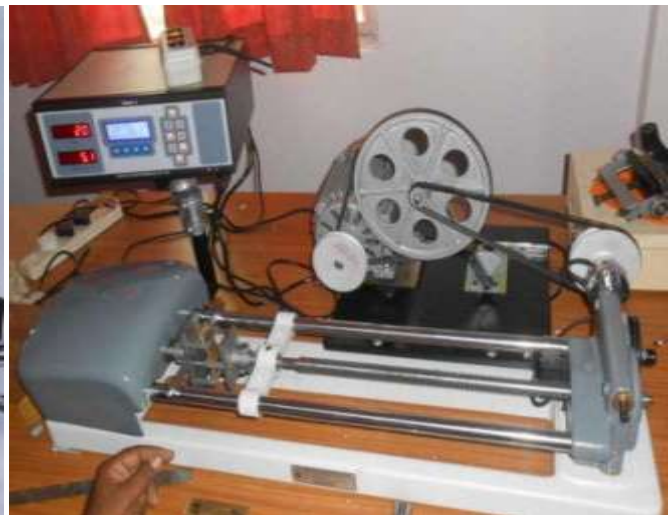
Fig.9 Electronic Tensometer for flexural testing of composites
