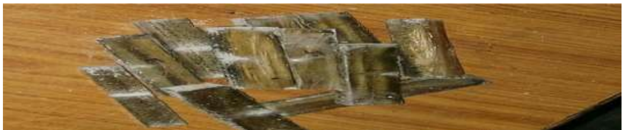
Fig.7 Impact testing specimens
