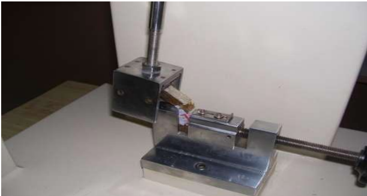
Fig.10 Composite under impact testing
