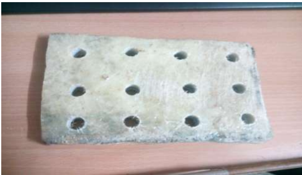
Figure 7 Drilled work piece based on Taguchi L 9 Orthogonal Array
