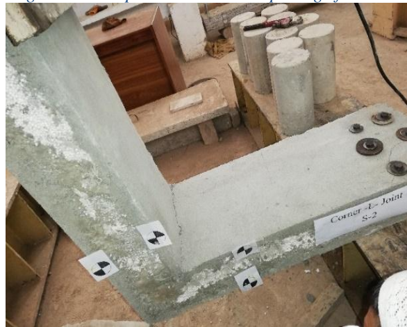
Figure 8. Joint Crack at the perpendicular walls
