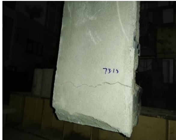
Figure 7. Back portion crack and spalling of concrete
