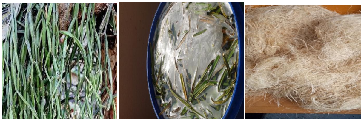
Fig.1 (a) CQ Plant, (b) CQ enzyme retting process, (c) Enzyme retting extracted CQSF.
