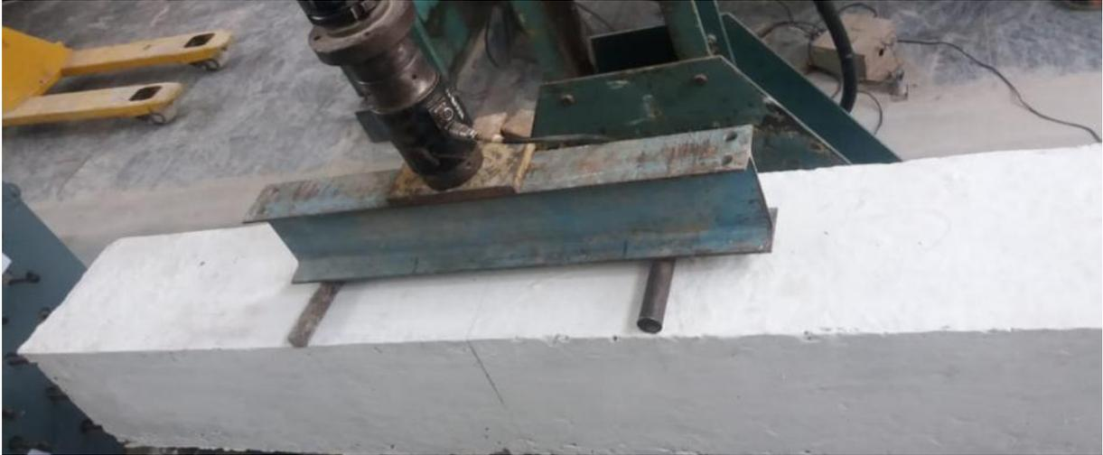
**Figure 4. Test Setup for testing controlled specimen**
