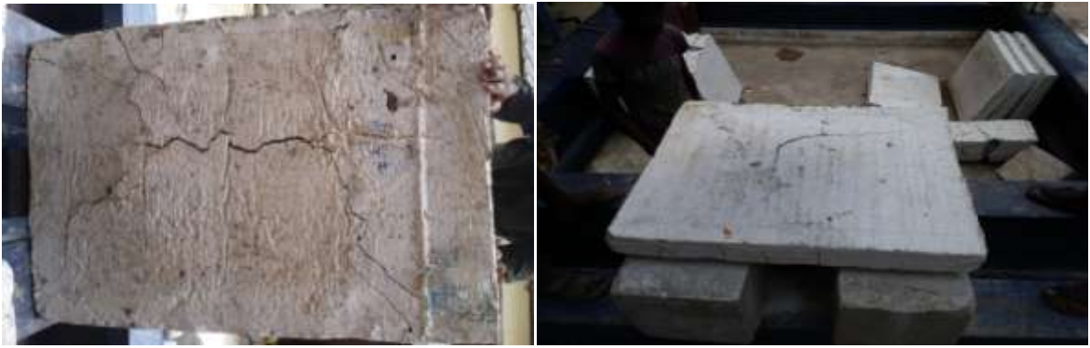
Figure.5 Failure profile after reaching ultimate load
