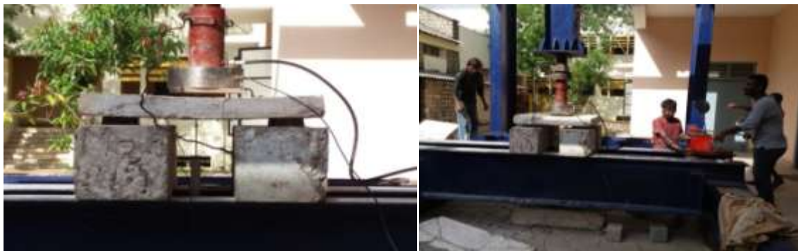
Figure.2 Test setup and application of load on the specimen
