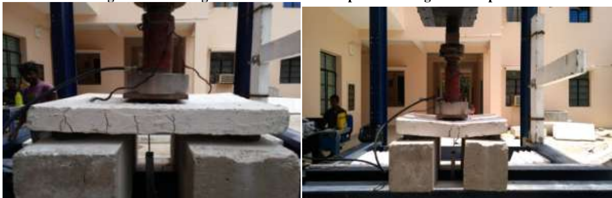
Figure.4 Crack propagation and ultimate failure of the specimen
