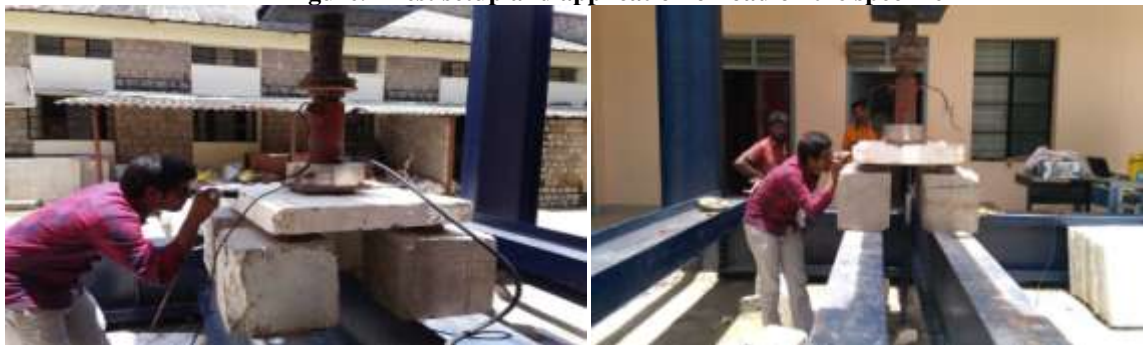
Figure.3 Observing the crack width of the specimen using crack scope
