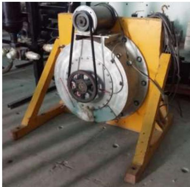
*Figure 3: Eccentric Mass Vibrator at Earthquake Engineering Center, UET Peshawar*
