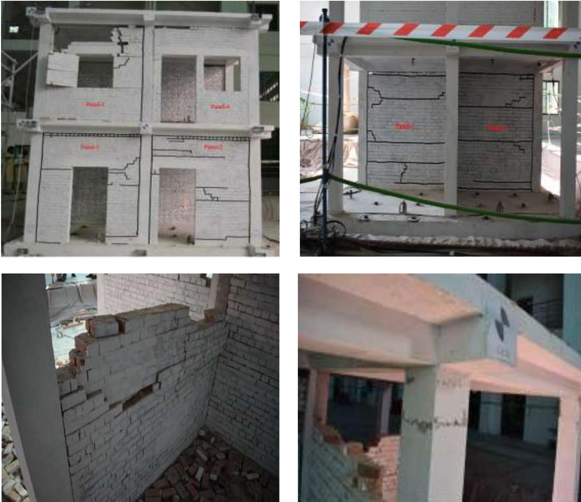
*Figure.2: Damage photos of test model*
