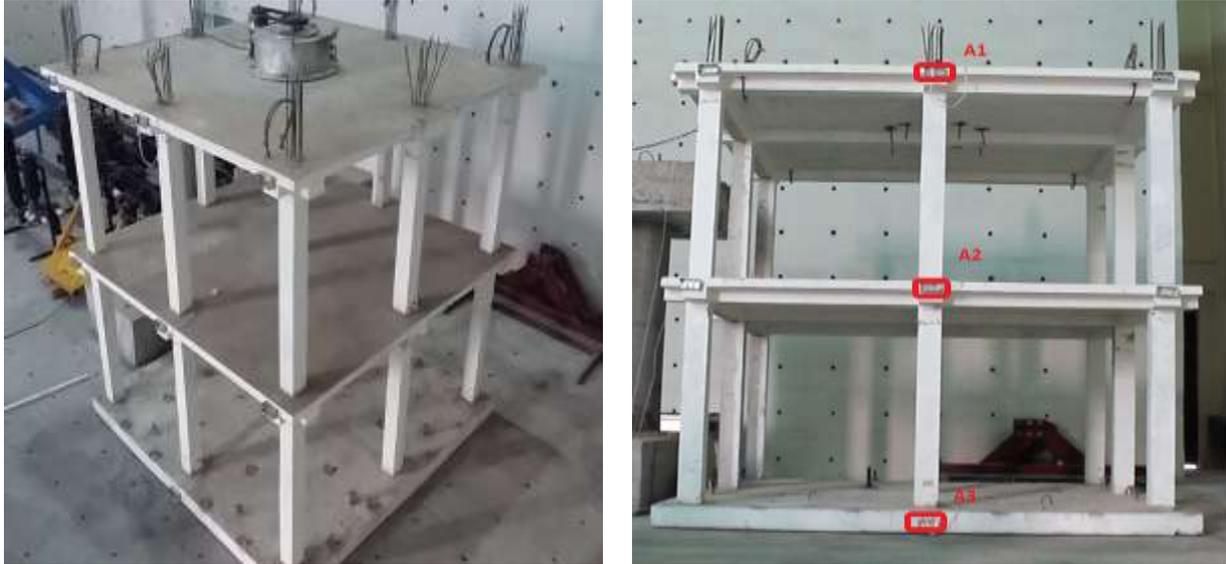
*Figure 4: EMV mounted on model (left), instrumentation of model (right)*
