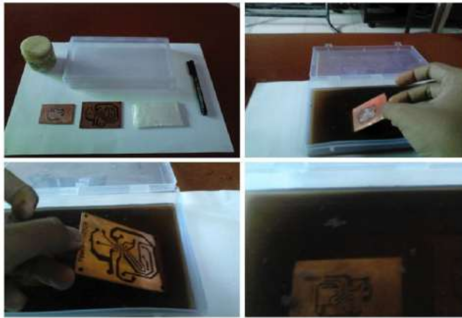
Figure 8: Rubbing away the oxide layer
