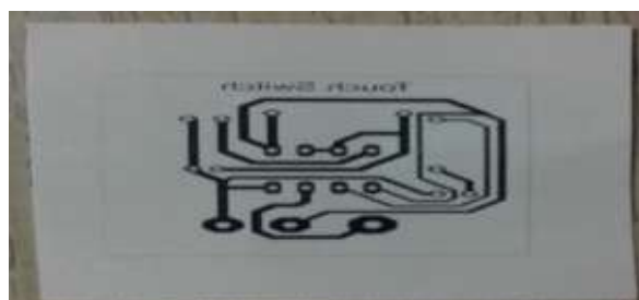
Figure : PCB print on Glossy side of paper
