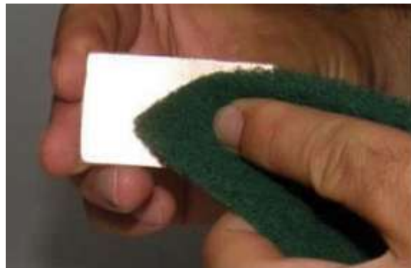
Figure 7: Rubbing away the oxide layer
