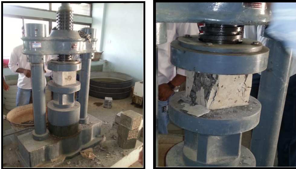
Fig 5: Compressive Strength Test
