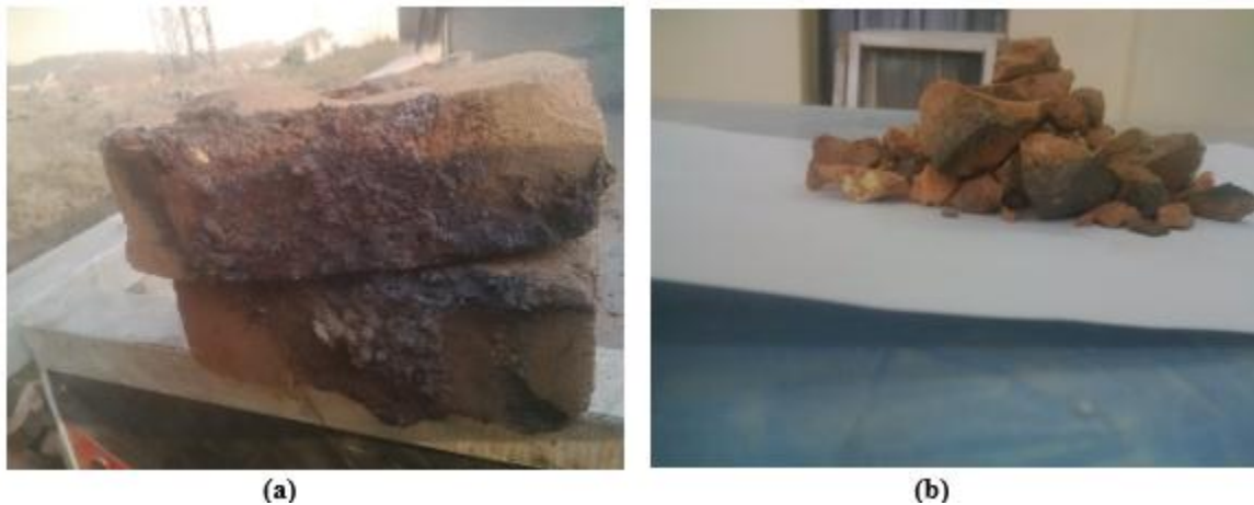
Figure 1: Over Burnt Bricks
